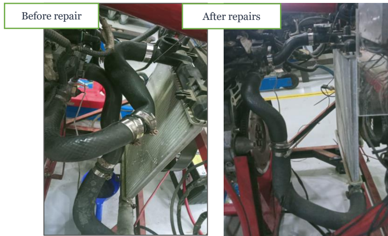
Figure 2. Comparison of Radiator Inlet and Outlet Hose Configurations Before and After Repair
