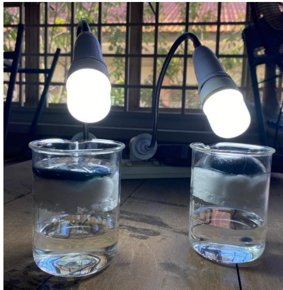
Figure 5. Evaporation experiment used a solar simulator lamp in three conditions 1-hour,12-hour continuous irradiation.
